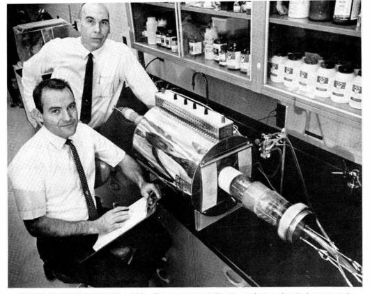
VAPOR PHASE GENERATOR, which offers great versatility in producing chemical compounds and mixtures, was recently patented by the AEC in the names of inventors Jim Corll (5316), back, and Dick Baughman (5154).
